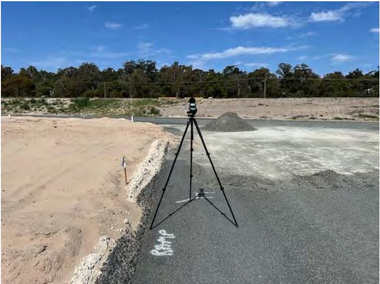
Figure 3-2: Photograph of Sound Level Meter on Site
