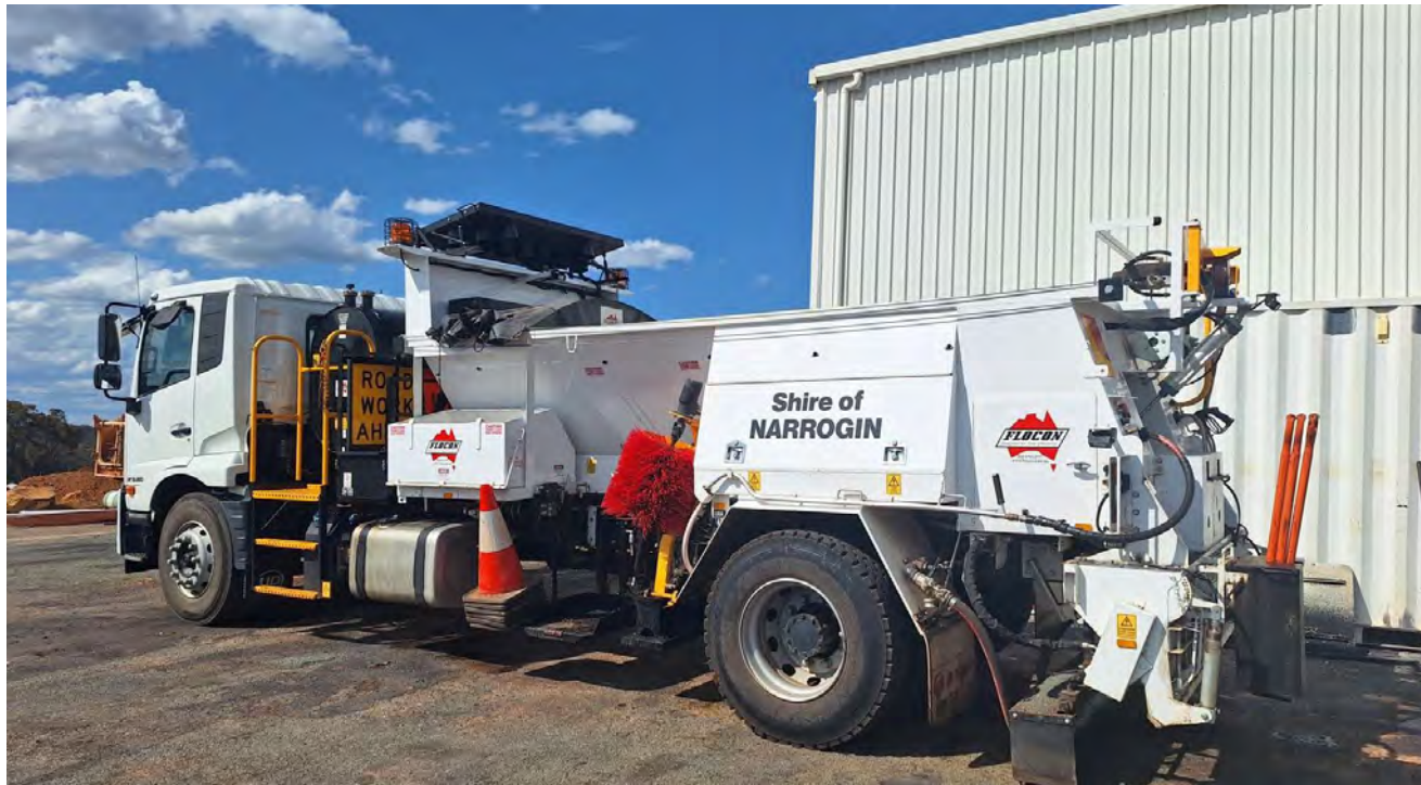
THE SHIRE OF NARROGIN'S ROAD DEFECT FLOCON UNIT
