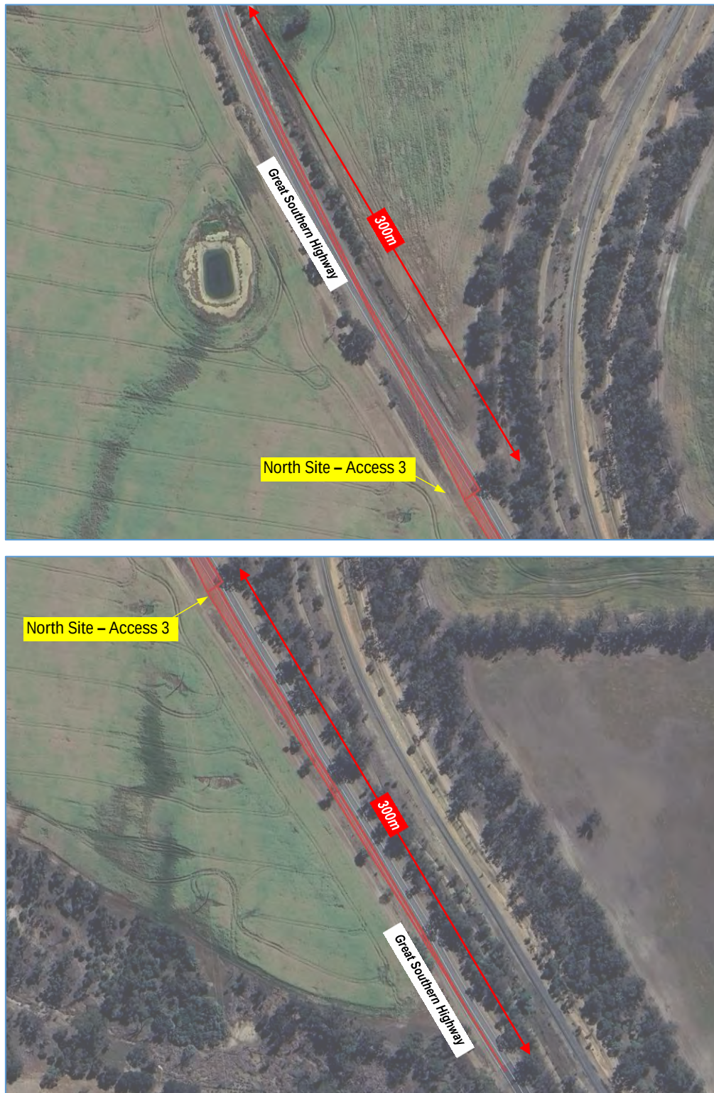
Figure 16: Northern Site Access 3 - Available Sight Distance
