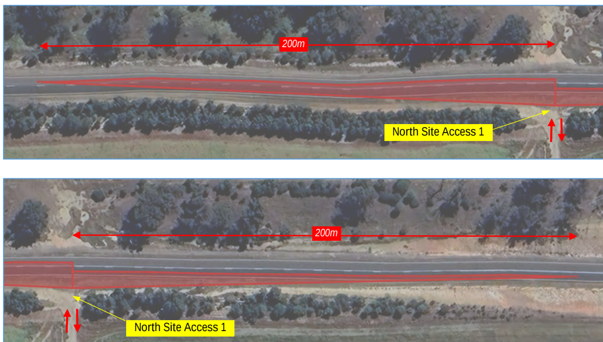
Figure 14: Northern Site Access 1 - Available Sight Distance
